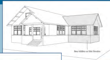
Side/rear addition placement
